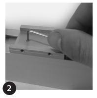
Position slider over plates (lock slider with grub screw/hex key).
