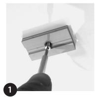
Check product/plate orientation and cable grommet clearance from mounting surface. Mark position of plates (supplied with the preinstalled sliders - 2 per metre).
