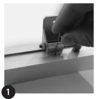
Secure brackets with hex key. Mark and drill holes for screws.
